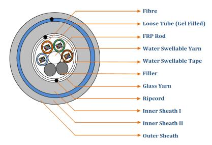
48 fibre cable shown. Other fibre counts are of similar construction.
